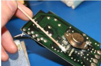
*Figure 36: Re-Clean the Desoldering Area*
