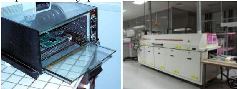
*Figure 29: Soldering Ovens*
