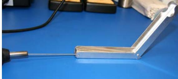
*Figure 8: Using the Desoldering Iron Cleaning Tool*
