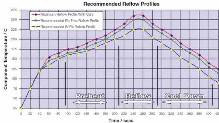
Figure 30: Typical Oven Program for Ceramic Capacitors
