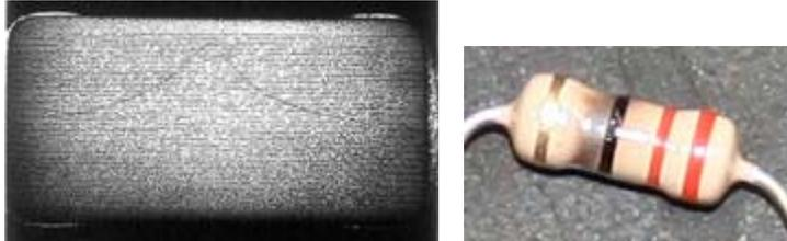
*Figure 19: A Crack in a Ceramic Capacitor and a Burnt Resistor*
