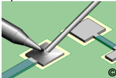
*Figure 32: Adding Solder to One SMT Pad*
