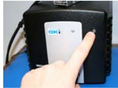
*Figure 24: Power Button on the OKI Soldering Station*
