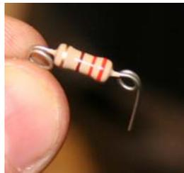
*Figure 17: Coiled Resistor Leads to Reduce Vibration Shearing*
