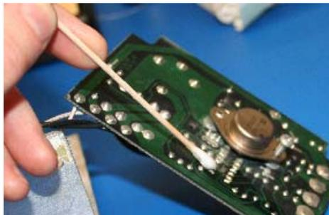
*Figure 23: Re-Clean the Desoldering Area*
