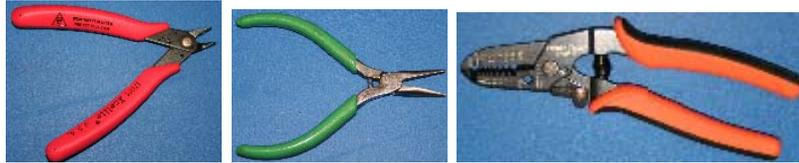
*Figure 13: Side Cutters, Needle Nose and Wire Strippers*
