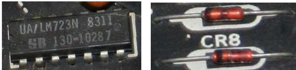
*Figure 4: Example of DIP16 and DO-35 Packages*
