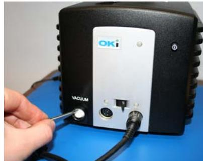
*Figure 8: Changing the Filter in the Desoldering Iron*
